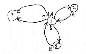
The numbered circles represent the *states* of the machine. At any moment the machine is in a particular state. The machine reads words, one letter at a time. If the machine is in some state, and sees a certain letter, it follows the arrow from its state with that letter as its label, and ends up in a new state. For example, if the machine above is in state 1 and it sees the letter B, it goes into state 3.
