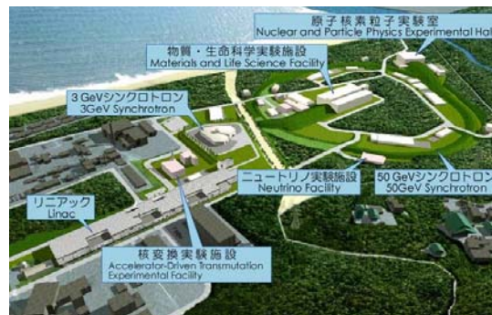
Figure 5.6. The J-PARC Facility at Tokai currently under construction. Its 3-GeV and 50-GeV high-intensity proton beams will drive a spallation neutron source and intense neutrino and meson sources. It will become operational before the next decade.
